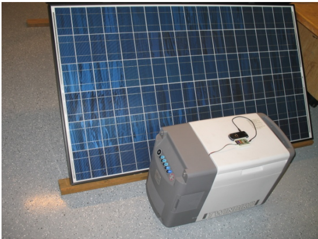
Figure 6: Solar-powered Cold-box Enhanced with Temperature Monitoring
