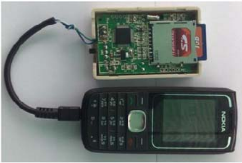
Figure 4: FoneAstra connected to a Nokia 1650 phone
