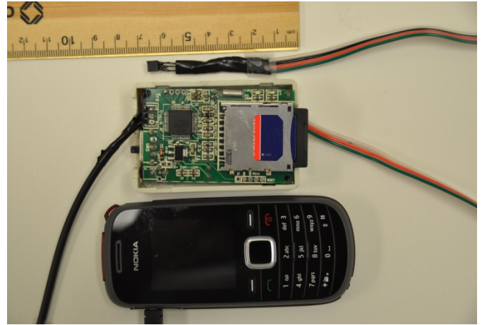
Figure 7: FoneAstra Enhanced with a Temperature Sensor Connected to a Nokia 1661 phone
